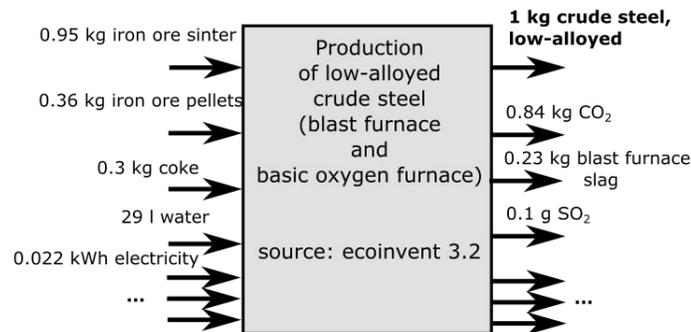
**Figure B1R1.4:** Three possible descriptions of a steel mill. a) A photo of a steel mill showing a blast furnace and heat exchangers. b) Schematic of the steel making process chain. c) A process inventory for steel making from a life cycle database. Each process representation serves a specific purpose, none of them is complete, but all contribute to a comprehensive depiction of the steelmaking process. [http://www.ushamartin.com/wp-content/uploads/2014/04/Process-flowsheet.jpg]
